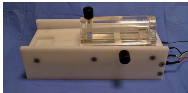
Fig. 1 Photograph of the six-lead restrained ECG monitoring system formed by a platform with ECG sensors and a size fitting half-tunnel
